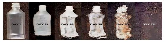
Bioplastics are plastic polymeric materials, obtained from raw materials of biological origin, that is, from renewable natural sources, such as biomass of starch, cellulose, lactic acid, fats, and vegetable and animal proteins, among others. The term bioplastics are used to distinguish these materials of biological origin, from petroleum plastics, which are made from petroleum derivatives.
